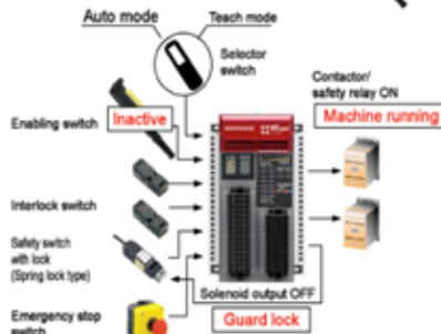
Teach mode (operating mode) - Machine running
