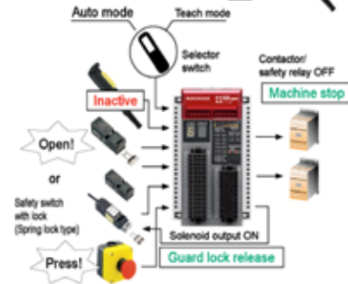
Machine stop (Safe state)
