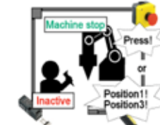
Machine stop (Safe state)
